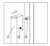
Locate the handle ① over the fixing pins ③ of the door and using the supplied allen key, tighten the securing grub screws ② to fix the handle.
